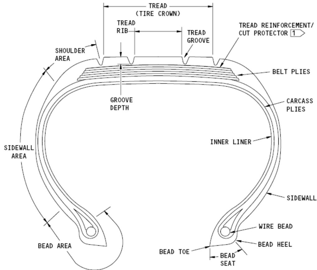
1 THE TREAD REINFORCEMENT/CUT PROTECTOR CAN BE METAL OR KEVLAR.
