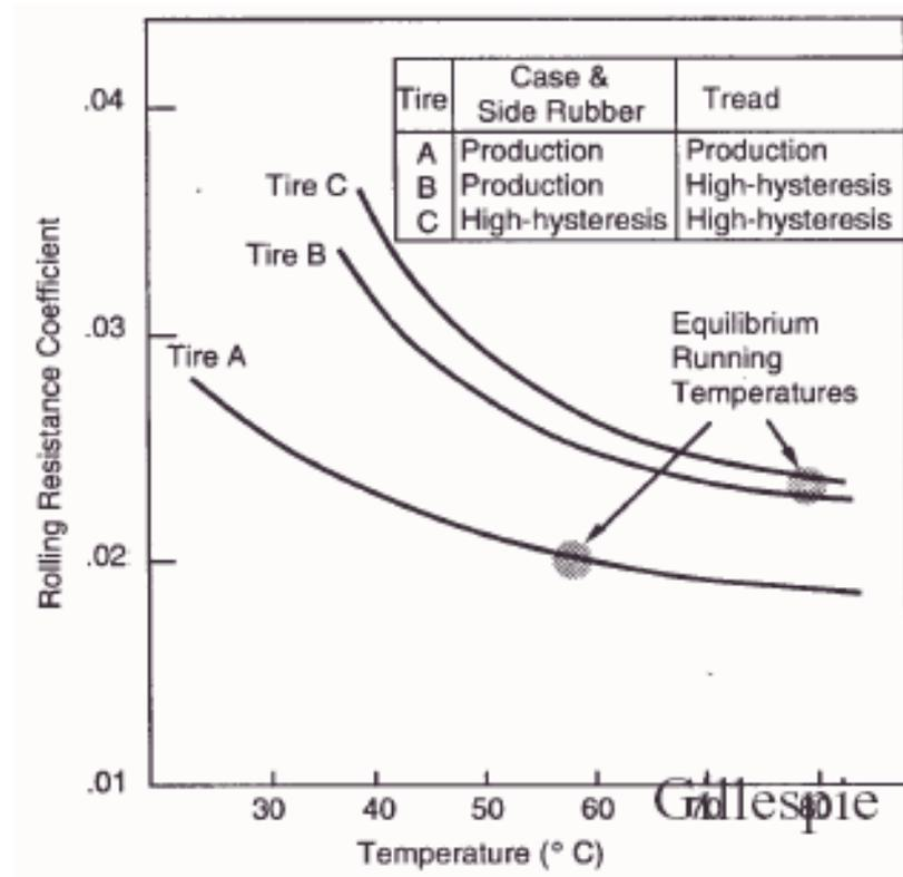
Gillespie Fig. 4.32 : Influence of the rubber quality, dissipation rate and working temperature
