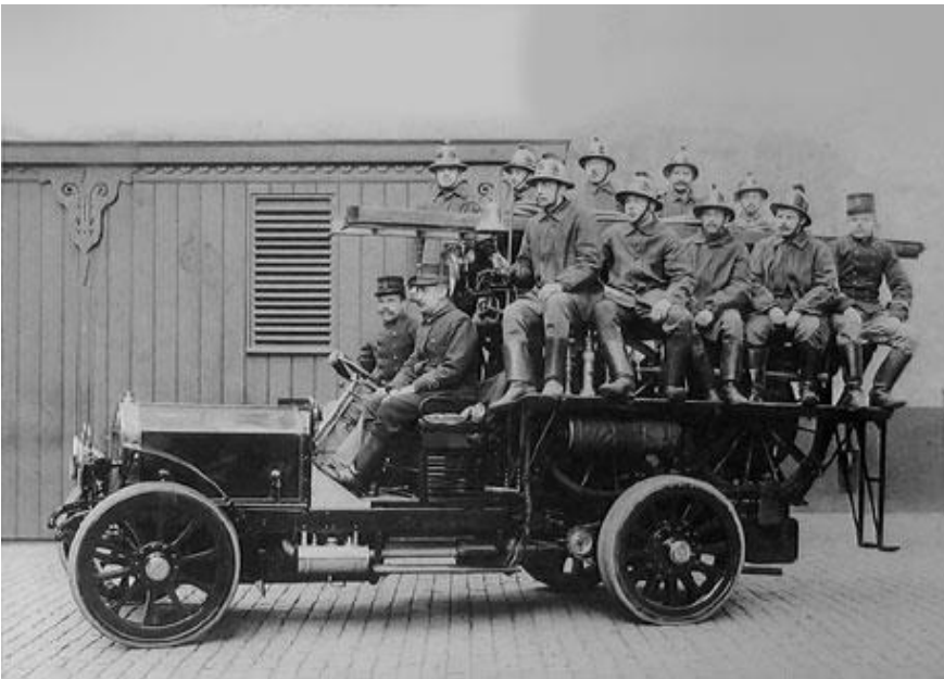
Pieper hybrid truck for Antwerp firemen (1912)
