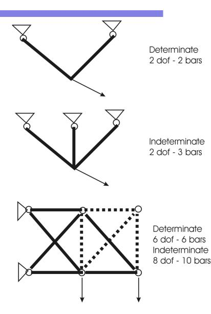
Statically determinate structures
