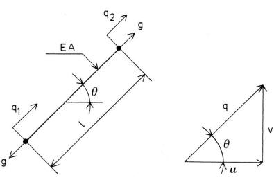
$$\begin{bmatrix} q_1 \\ q_2 \end{bmatrix} = \begin{bmatrix} \cos \theta & \sin \theta & 0 & 0 \\ 0 & 0 & \cos \theta & \sin \theta \end{bmatrix} \begin{bmatrix} u_1 \\ v_1 \\ u_2 \\ v_2 \end{bmatrix}$$
