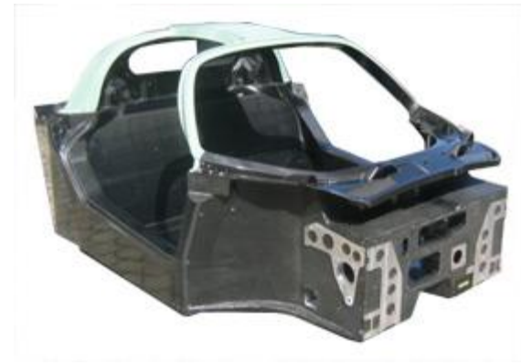
Composite monocoque chassis Ferrari Enzo
