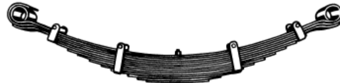
a. Conventional multi-layer leaf spring with smoothly cut layer-ends. 14 layers; height of bundle: 140 mm; weight: 122 kg
