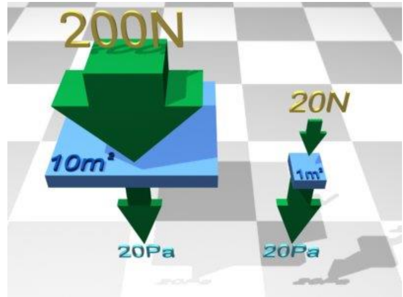
Hydraulic system with different pistons surfaces
