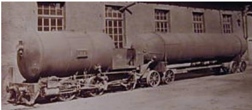
Pneumatic locomotives, during the construction of the Gotthardbahn from 1872 to 1882
